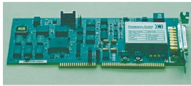
MACEAS ultrasound module with digital signal processor
